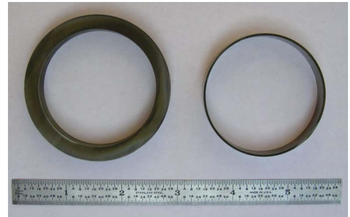
MA956, starting tube 0.25" thick wall. flow formed tube 0.03-0.04"
